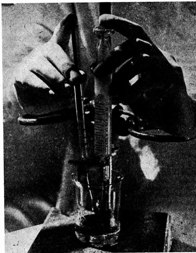
Fig. 11. Apparatus used for labelling of the blood serum proteins with radioactive iodine.
